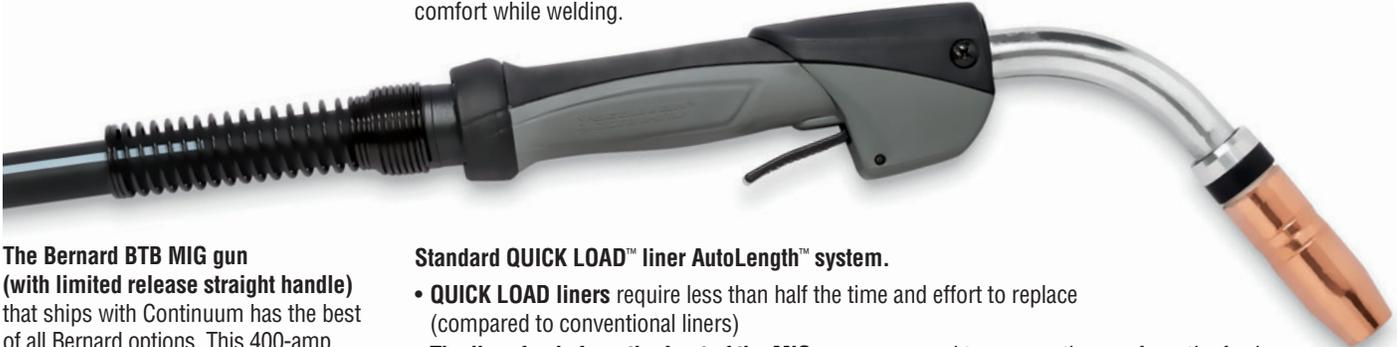
The Bernard BTB MIG gun (with limited release straight handle) that ships with Continuum has the best of all Bernard options. This 400-amp, air-cooled MIG gun is recommended for heavy manufacturing environments.
