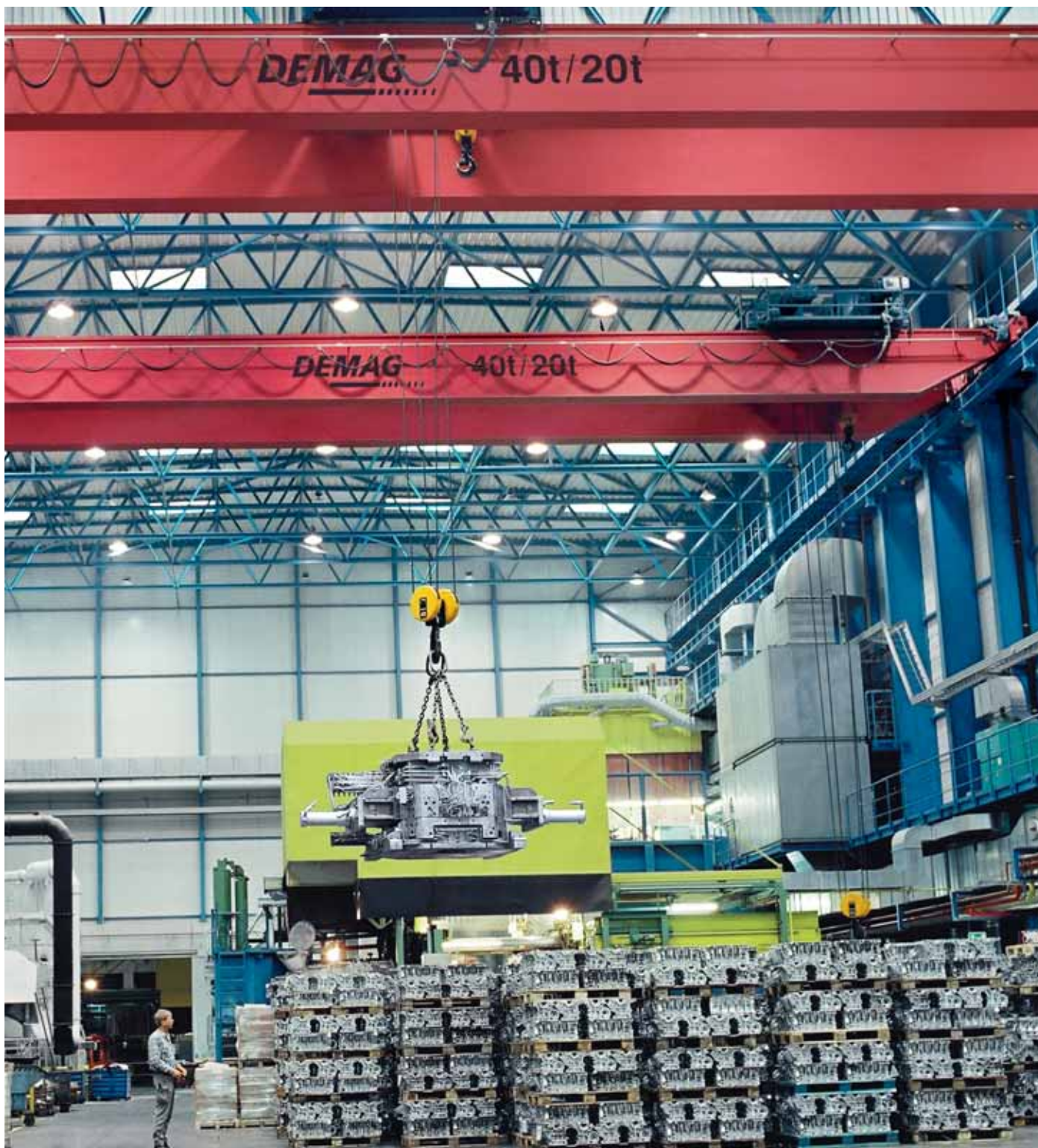
Double girder overhead traveling crane with tandem end trucks for transporting and turning engine blocks
